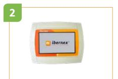
Touch screen and RFID scanner to code tasks and alarms answered. Consultation of tasks pending, room presence log via RFID scanner or touch screen and coding of the tasks and alarms answered.
