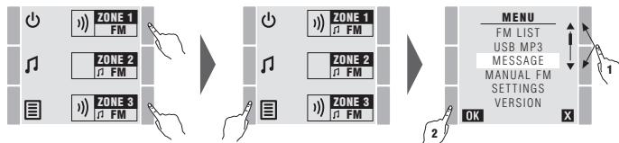
When the **MESSAGE** option is entered the system also searches the root directories on the SD micro card. While this operation is performed an hourglass appears on the screen for several seconds.
