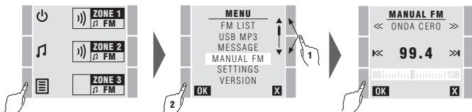
To select and listen to the 30 preset stations, select the required radio station as follows. It will be available in the zones for which **FM** has been selected.
