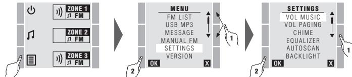
The zone selection screen is displayed and one zone can be chosen to change the volume or ALL of the zones can be selected to apply the change to all of the zones at the same time.
