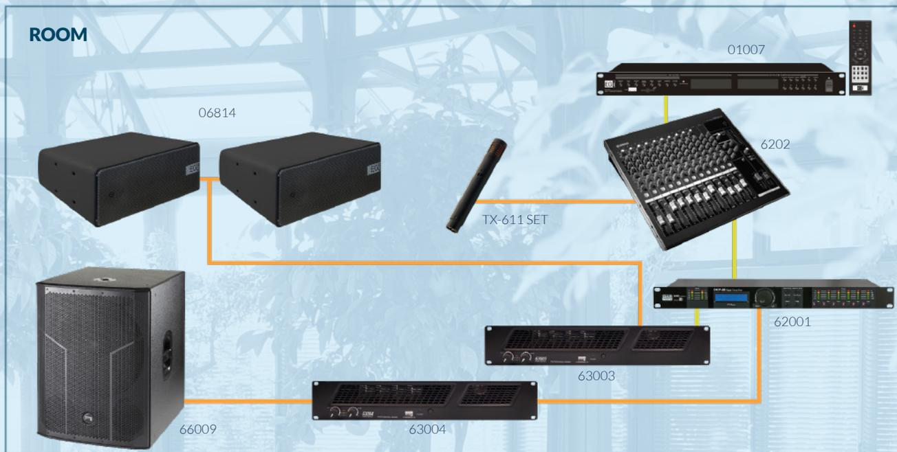
The example above is an example of a professional installation for a party room with 2 stages, one for subwoofers -66009- and another one for the line arrays -06814- and the mixing console with microphone and music source.
