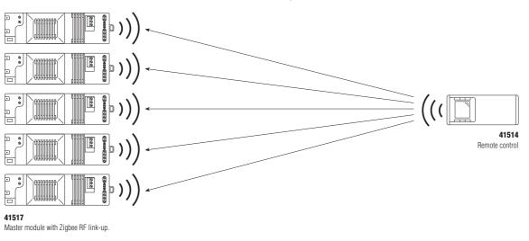
MAXIMUM MULTIROOM LINK-UP OF 41517 MASTER MODULES, THROUGH ONE 41514 REMOTE CONTROL
